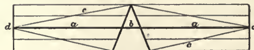
FIG. 42.—Wenham's system of Aeroplanes designed to carry a man, a, a , Thin planks, tapering at each end, and attached to a triangle. b , Similar plank for supporting the aeronaut. c, c , Thin bands of iron with truss planks a, a , and d, d , Vertical rods. Between these are stretched five bands of holland 15 in. broad and 16 ft. long, the total length of the web being 80 ft. This apparatus, when caught by a gust of wind, actually lifted the aeronaut.
